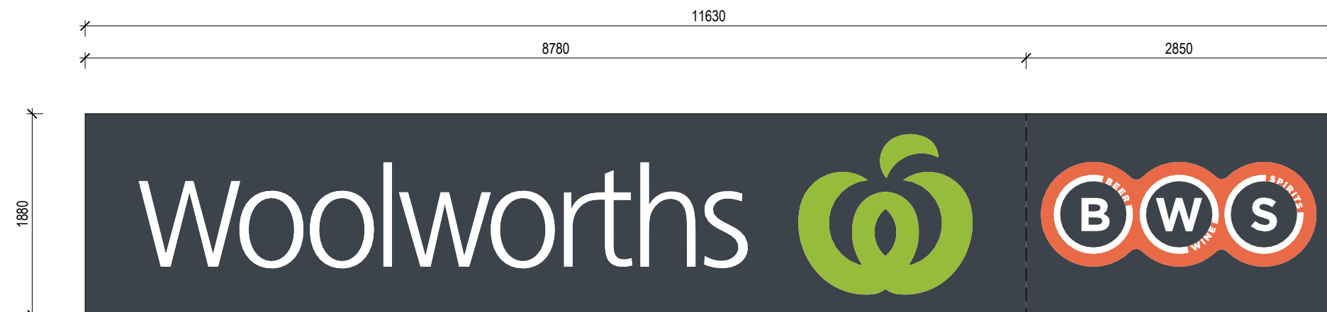
S 2.1 EXTERNAL FACADE SIGN COMBINED SIGN 11630mm x 1880mm OVERALL. (1500mm HIGH WW LOGO) INTERNALLY ILLUMINATED SIGN. MOUNTED TO FACADE OF BUILDING. REFER SIGN B11 IN WOOLWORTHS SIGNAGE DESIGN BRIEF 2021.1 (Rev. E)
